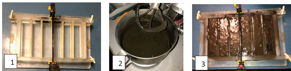
Figure 2. 1 - A Plexiglass mould, 2 - The mixture, 3 - The mixture placed in the mould/ Rysunek 2. 1 - Forma z Plexiglass, 2 - Mieszanka, 3 - Mieszanka w formie
